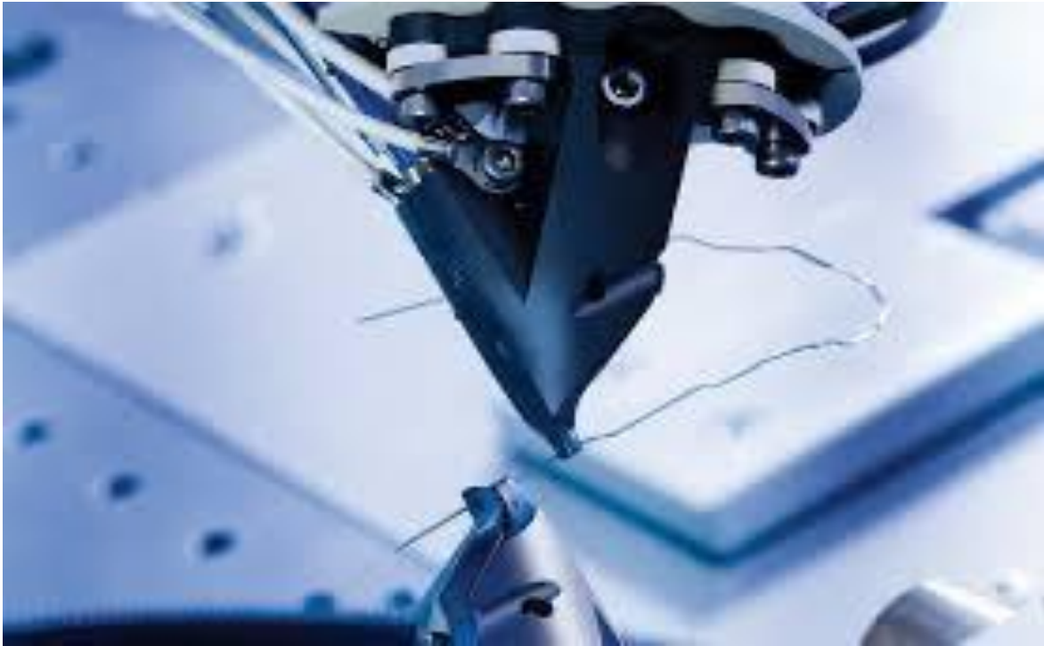
Figure 3 Machine processing model consisting of two robotic arms equipped with pliers for bending the archwire with perfect accuracy and precision.
